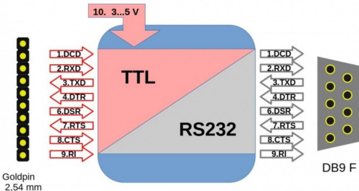
On the converter board, on the lower description layer, there are precise markings for each signal on each connector:
